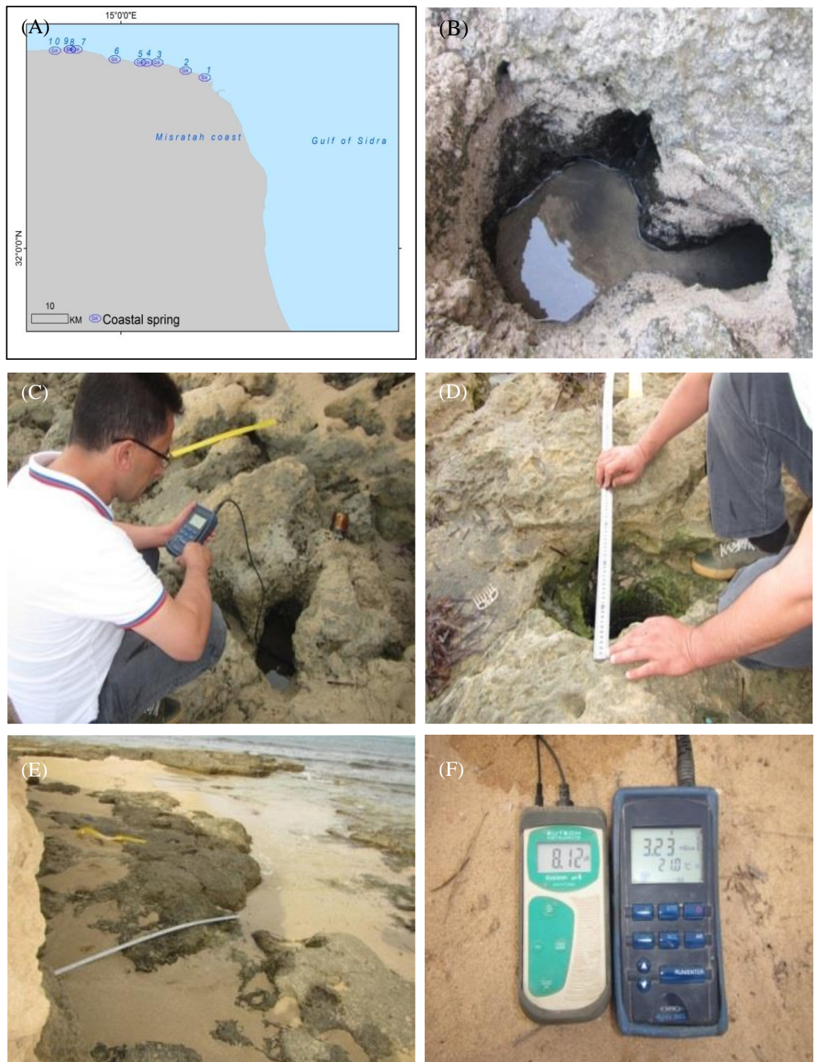
Figure 19 (A) Coastal freshwater spring distribution on the north coast, (B) shows egress of groundwater during the measurement, (C) recording characteristics of the coastal aquifer in summer, (D) measuring the dimension of the well hole, (E) coastal spring located in the intertidal area which is completely covered by seawater and sand, (F) types of equipment used in the field to determine the physicochemical parameters of the coastal spring water, (1) electrical conductivity (EC), (2) PH/ C meter.
