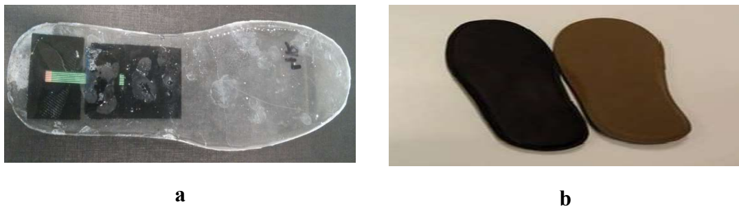
Figure 6.6: a) PCB components embedded in a clear 4mm polyurethane layer b) Top layer (black artificial leather) and bottom layer (Brown EVA Foam)
