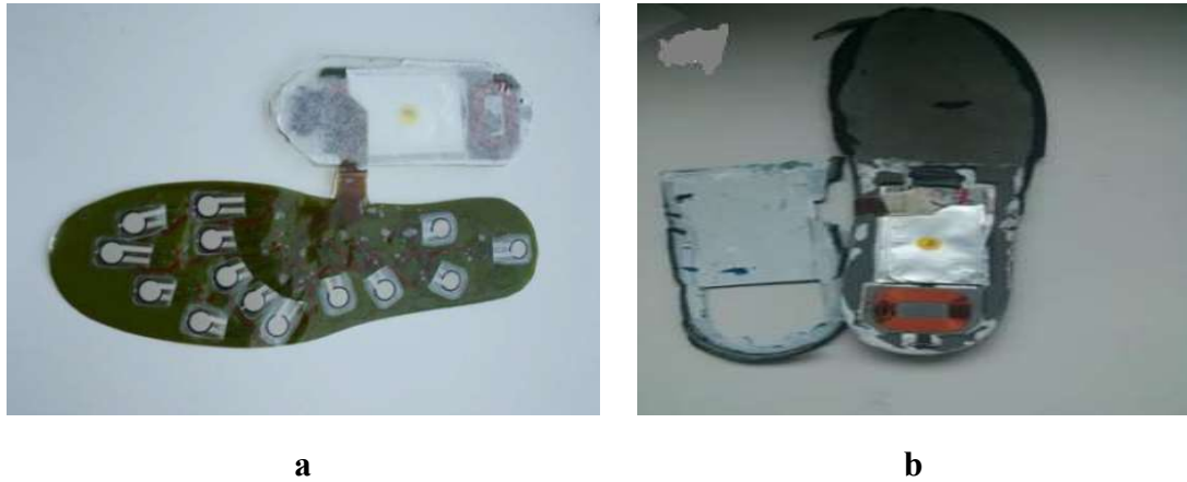
Figure 6.13: a) The clear polyurethane layer was removed to improve the flexibility of the insoles and the sensors were embedded in a thinner green Kapton (0.1mm versus 1mm for the previous sensor layer encapsulation); b) The PCB were now embedded in an expanded EVA foam layer 5mm
