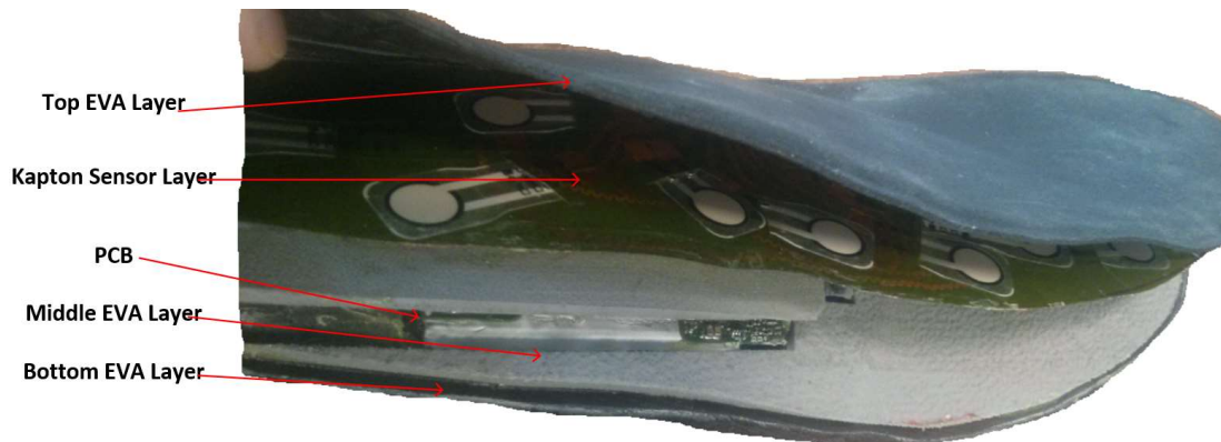
Figure 6.14: A cross-sectional view of the new version of the insoles showing the different layers from top to bottom
