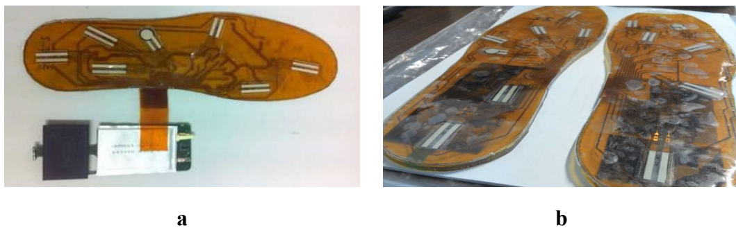
Figure 6.5: a) 1mm polyurethane sensor layer; b) Sensor and PCB layer glued together
