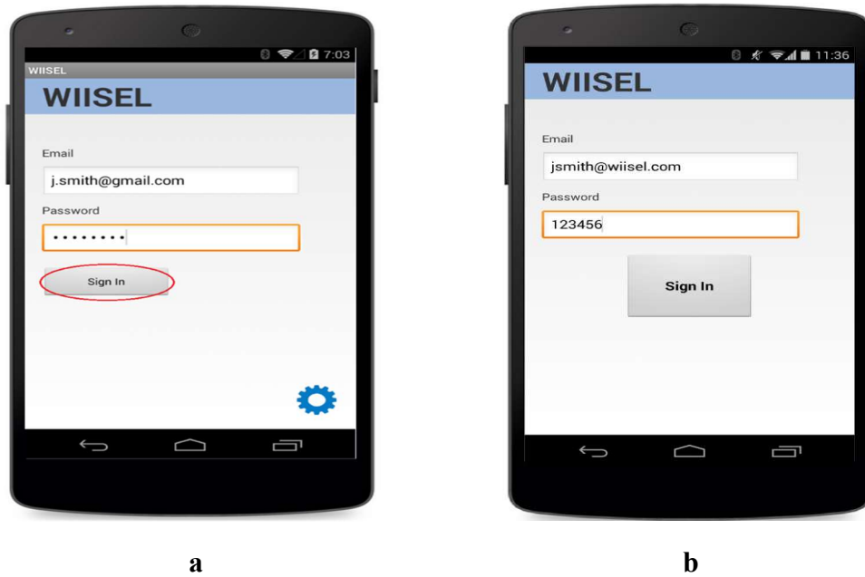
Figure 5.4: a) Experts were concerned with the small button size and the fact that the password was encrypted meaning an older adult might lose their place when typing. This problem was also identified by end users; b) Increased text size and a larger, more prominent Sign In button as well as a decrypted password
