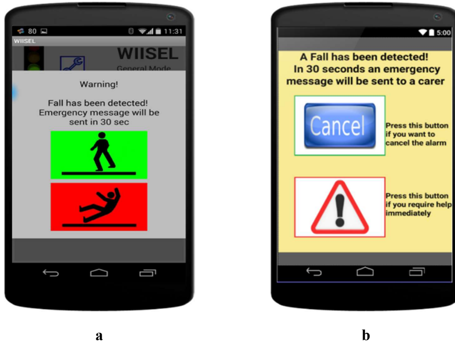
Figure 5.7: a) Fall Alarm Interface before Expert Inspection, the red and green caused confusion as the red was associated with ‘Cancel’ as you would find on a phone call interface; b) Fall Alarm Interface after Expert Inspection, a more appropriate symbol was introduced for the help button while the cancel button was changed to a more neutral blue with appropriate labelling
