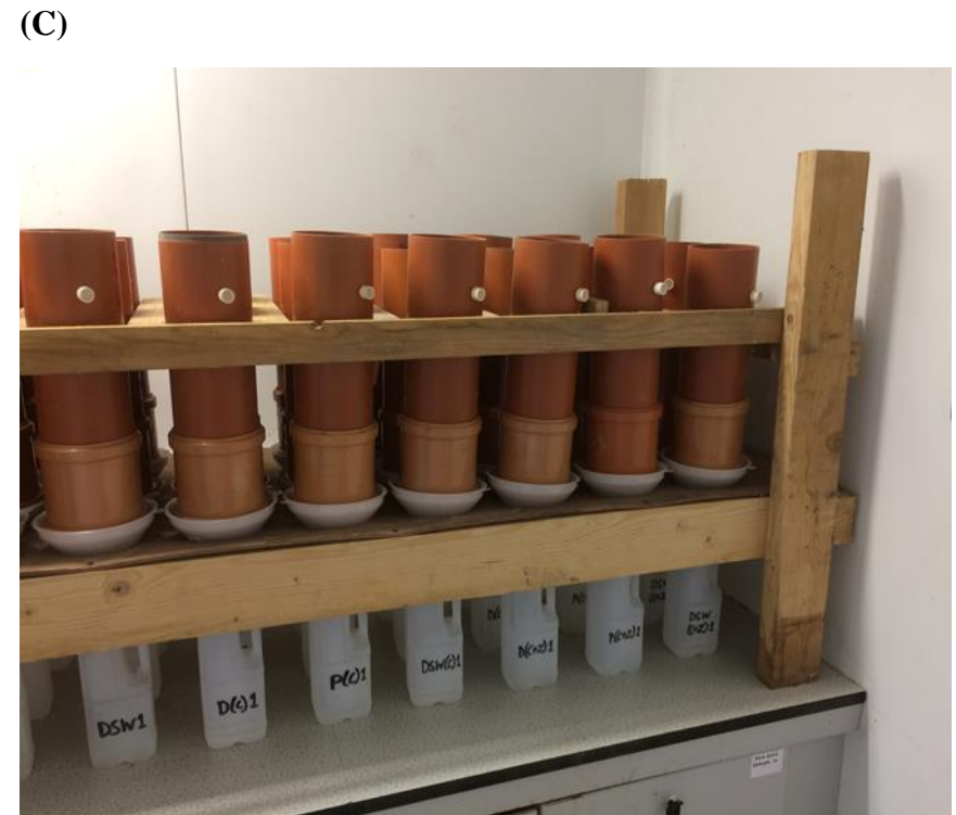
Figure 4.1 Schematic diagrams of typical column setup for leachate sampling (A) and column setup during gas sampling (B) (Not to scale). Image of laboratory set up during the experiment (C).
