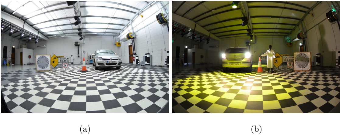
Figure 5.1: Two diorama scenes from vision laboratory: scene (a) is illuminated evenly with ambient white light of 86 lux; Scene (b) simulates street light illumination.
