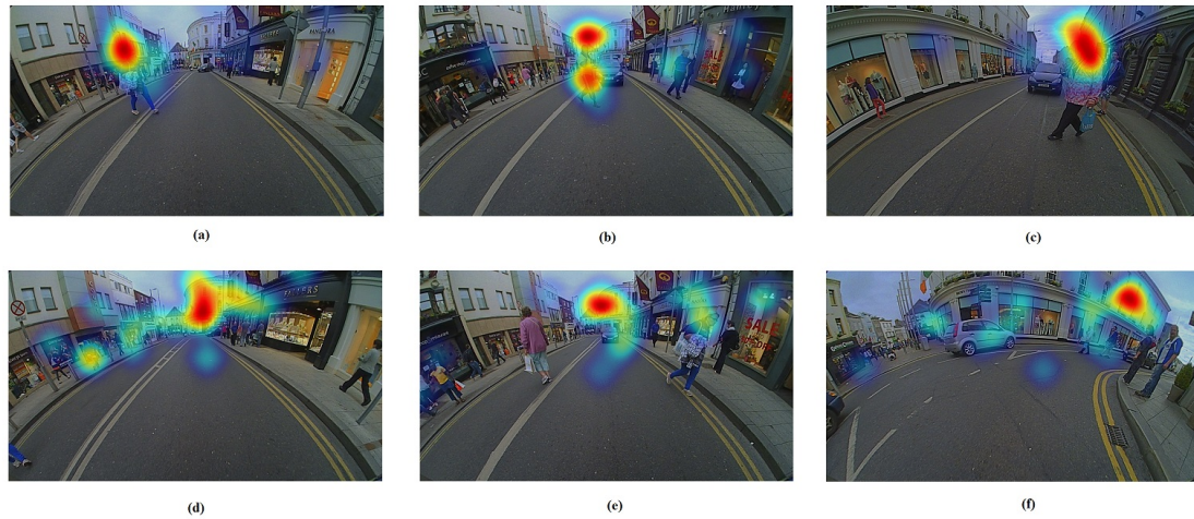
Figure 5.18: The frames with lowest inter-observer variability (a-c) correspond to frames with a single point of focus (a pedestrian), while frames with the highest inter-observer variability (d-f) contain multiple salient regions (many pedestrians or vehicles).
