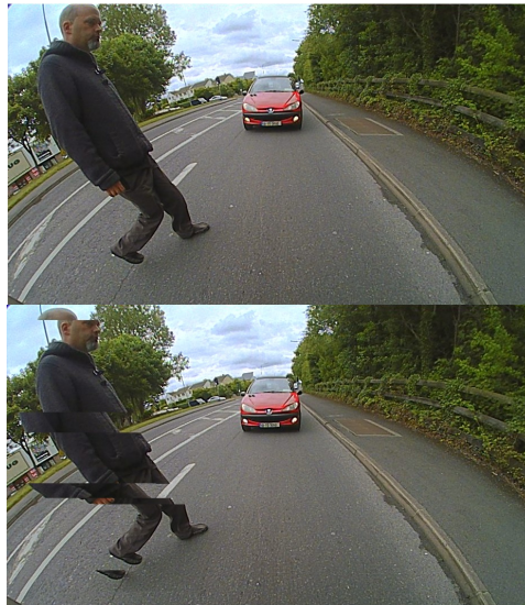
Figure 5.14: An input and extracted output frame from simulation after undergoing 10% packet loss.
