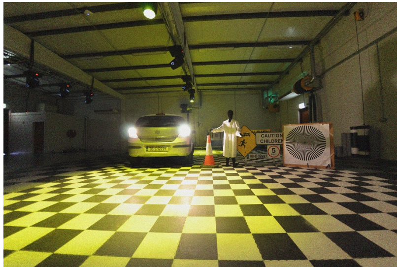
Figure 5.12: Example image taken in low light conditions. Thermal noise from the image sensor is the predominant distortion.
