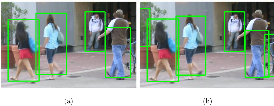
Figure 1.2: (a) Original clean image. “Ringing” caused by JPEG2000 (JP2) compression (b) can occur at high spatial frequencies which are difficult for the human visual system to discern, nonetheless the presence of this distortion is sufficient to degrade the performance of a pedestrian detection algorithm by causing an increase in false positives (indicated by spurious green boxes).
