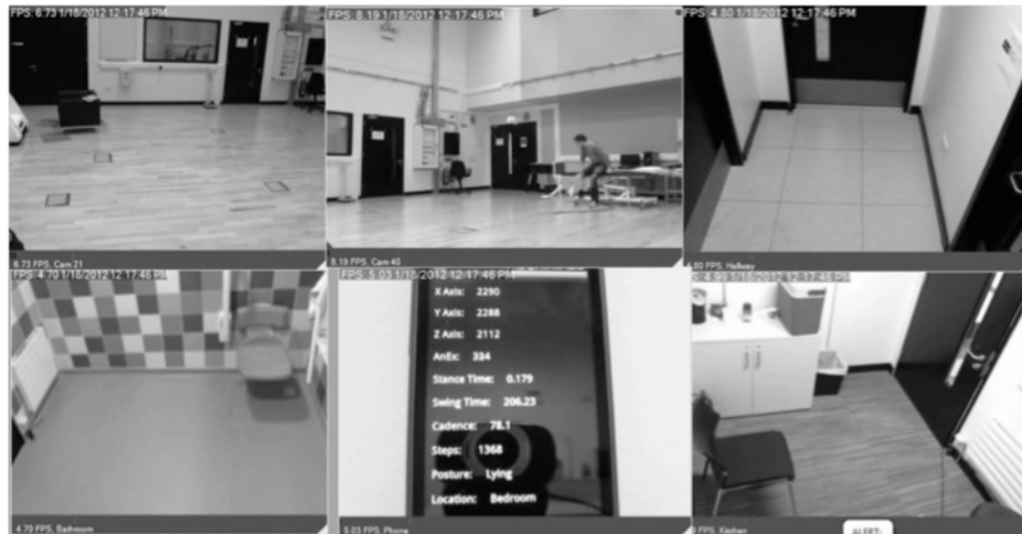
Figure 5.2: Camera output used to validate device output vs actual location and activity performed
