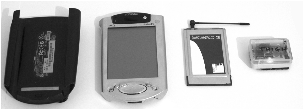
Figure 4.2: Pilot study apparatus showing from left to right: the external PCMCIA slot for interfacing the RFID reader to the PDA, the PDA, the RFID reader and the SHIMMER accelerometer platform used in the study
