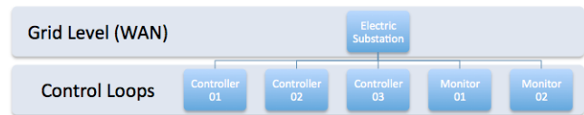
Fig 2(a): Legacy Electric Substation Architecture.
