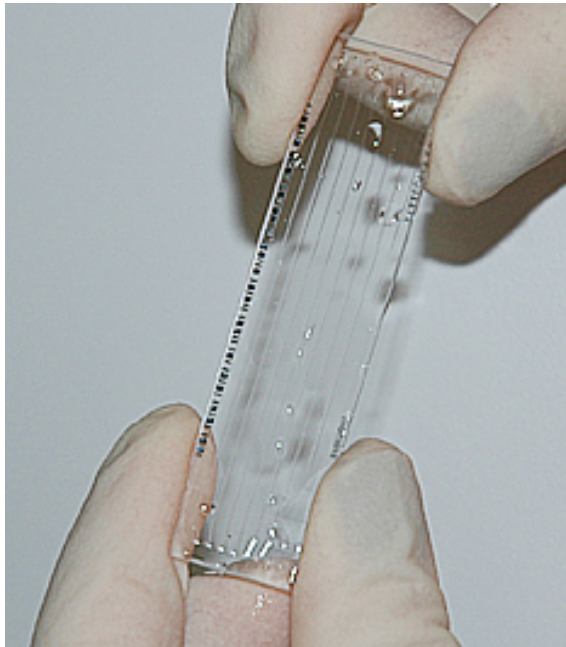
Figure 1.10: Photograph of an Illumina flowcell (sourced from [7]) and a diagrammatic representation of the millions of oligonucleotides present on the surface of the flowcell (sourced from [8]).
