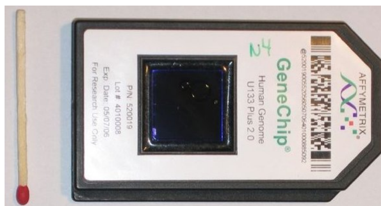
Figure 1.5: Affymetrix GeneChip microarray shown with a matchstick for scale. Sourced from [5].
