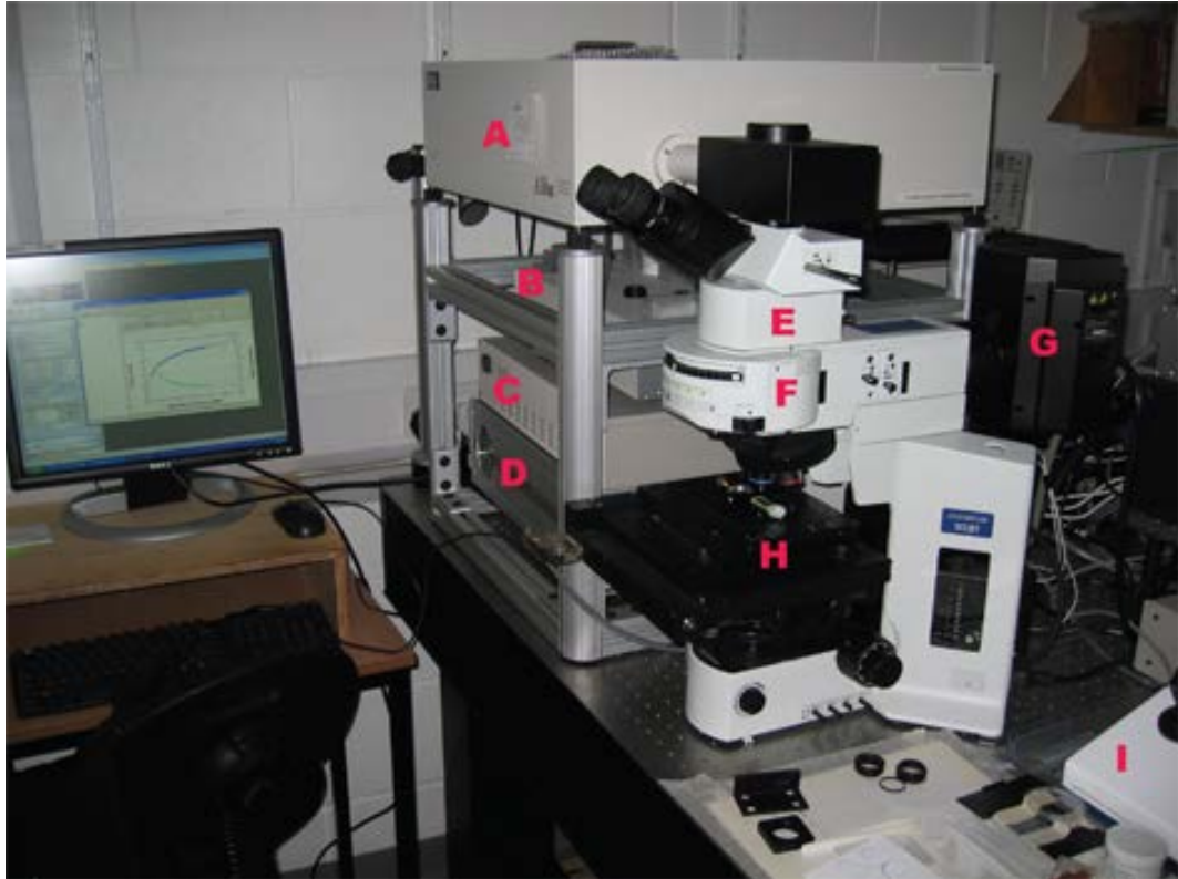
Figure 2.2: ISS Alba system. A: Detector unit. B: Synchronisation unit. C: RF amplifier. D: Dual frequency generator. E: dichroic mirror (separates excitation and emission light). F: filter turret. G: Widefield light source (Hg lamp). H: XY scanning stage and XYZ piezo electric stage. I: controller for XY scanning stage.
