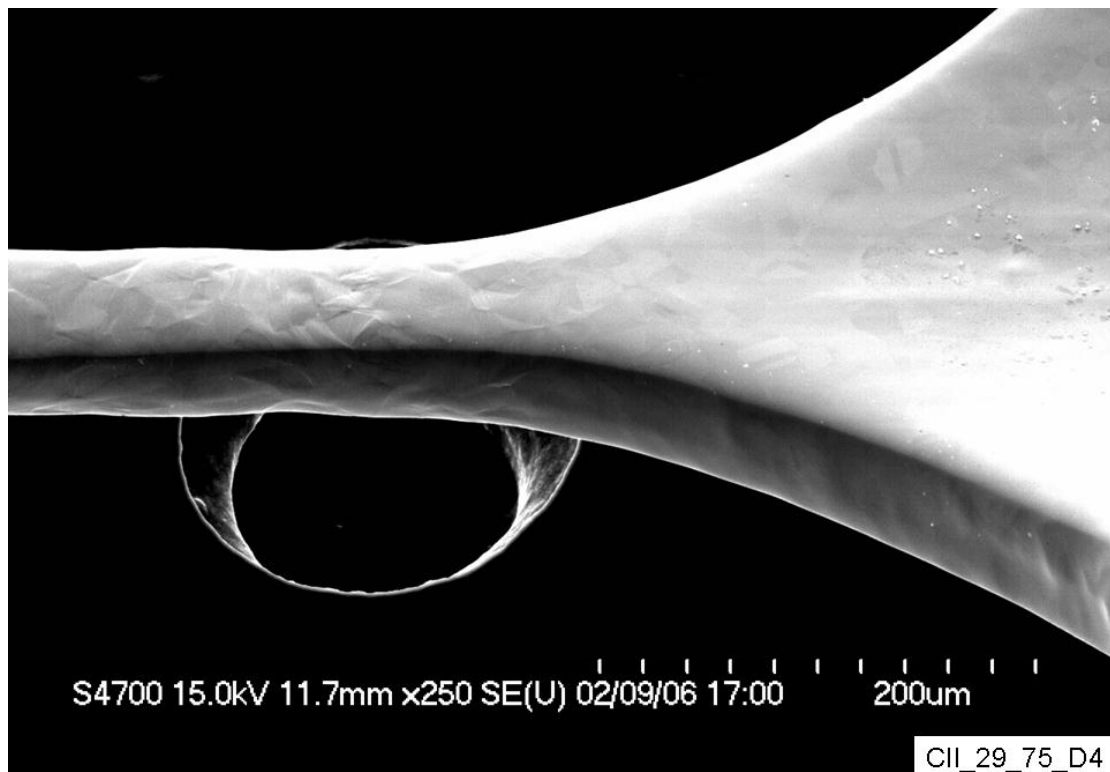
Figure 6.5. Plastic deformation within a 75 \mu\text{m} specimen; (a) heavily deformed region (b) comparably deformed region. Both images from same specimen.
