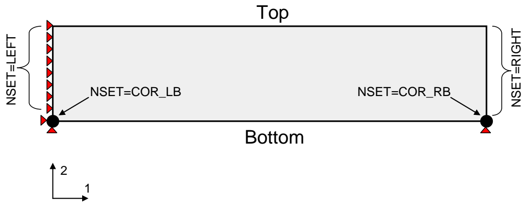
Figure 7.5. Schematic representation of boundary conditions for stand-alone struts. NSET is an ABAQUS abbreviation for “node set”.
