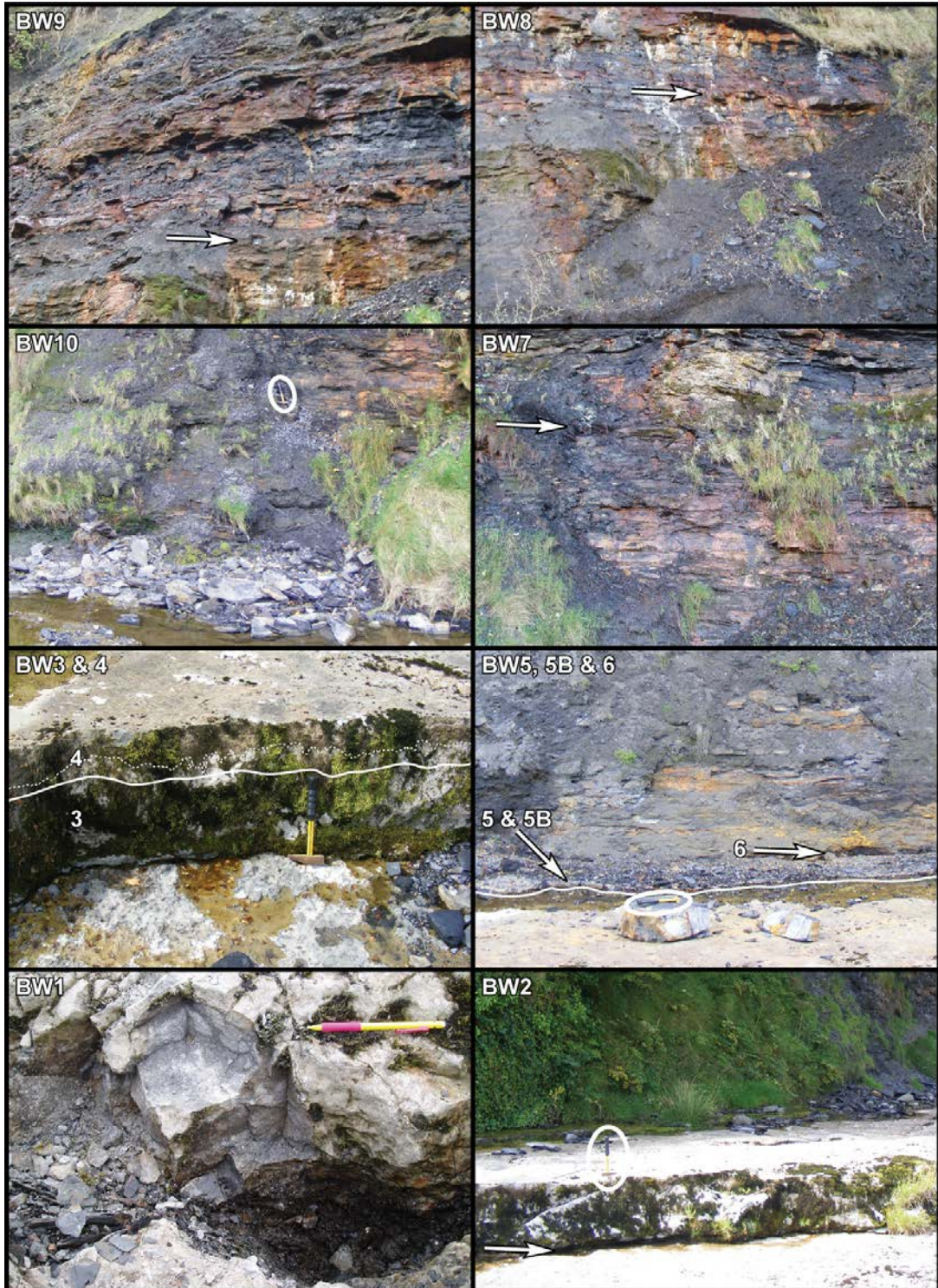
BW1 – The mechanical pencil points to where the bed was sampled within a joint in the bed surface, stream bed. BW2 – The white arrow indicates the location of the sampled horizon, in the overhang between prominent limestone beds, note the hammer (circled in white) for scale. BW3 & 4 – The hammer head marks the base of the sampled horizon BW3, whilst the solid white line defines its top. The upper portion of the bed was sampled as BW4, with the dotted white line marking the extent of probable phosphatisation. BW5, 5B & 6 – Numbers and white arrows indicate the horizons which were sampled. Note the hammer (circled in white) for scale. BW10 – The hammer (circled in white) sits on top of the sampled bullion horizon. BW7, BW9 & BW8 – White arrows indicate the sampled horizons, Fields of view are ~10-15m across.
