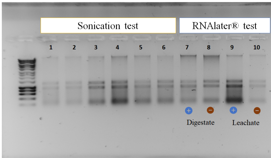
Figure C.3: Electrophoresis gel after the DNA/RNA co-extraction of samples testing different sonication times (1 to 6), and the use of RNAlater® in digestate and leachate samples.
