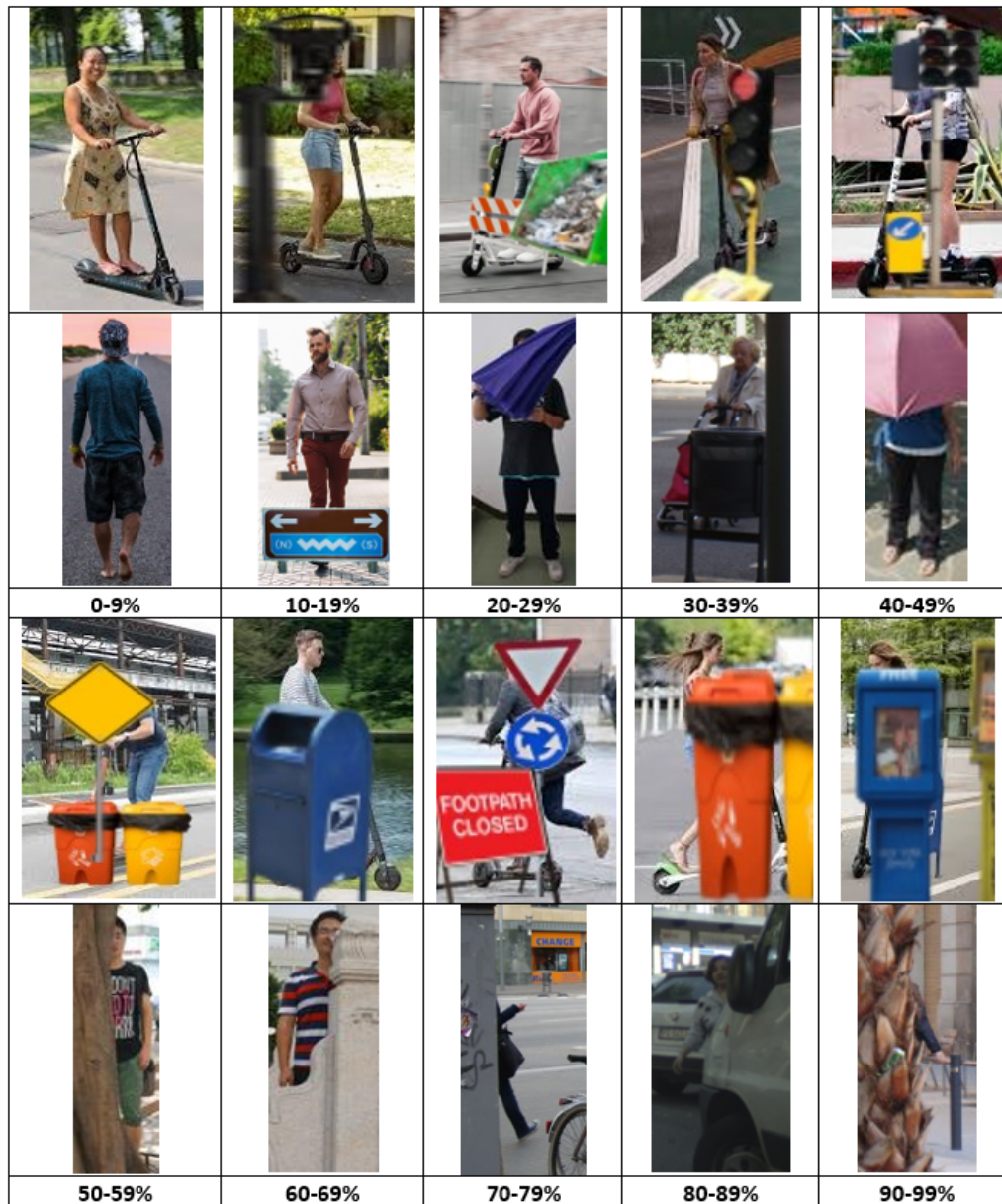
Figure 5.2: Test Dataset Sample. An example of dataset images for each level of occlusion. The custom dataset consists of 1,130 images, including 543 e-scooter rider images and 587 non e-scooter rider images.
