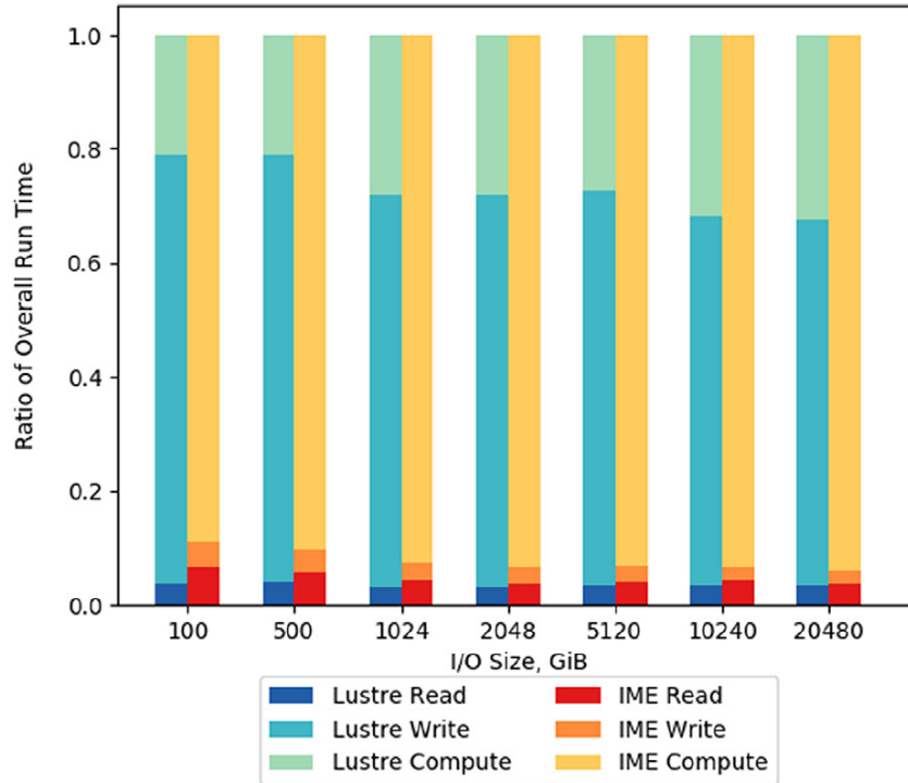
Figure 3.5: Fraction of runtime spent on IO and SEG-Y computations for LFS and LFS-supported IME. Reprinted from "ExSeisDat: A set of parallel I/O and workflow libraries for petroleum seismology" by Fisher, M.A., Conbhuí, P.Ó., Brion, C.Ó., Acquaviva, J.T., Delaney, S., O'brien, G.S., Dagg, S., Coomer, J. and Short, R., 2018, Oil & Gas Science and Technology—Revue d'IFP Energies nouvelles , 73, p.74 [1].
