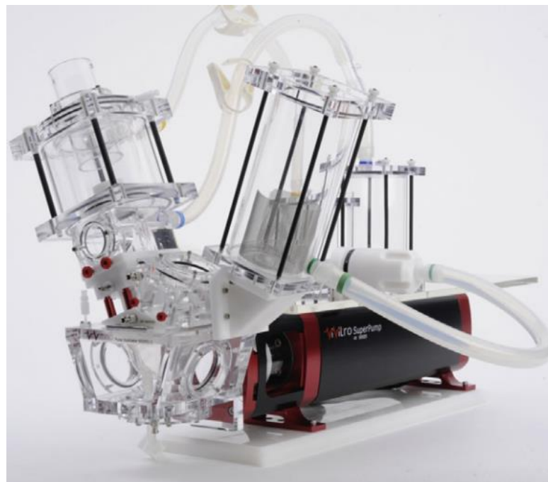
Figure 1.3 Vivitro Pulse Duplicator, adapted from Sathananthan et al. (2019)
