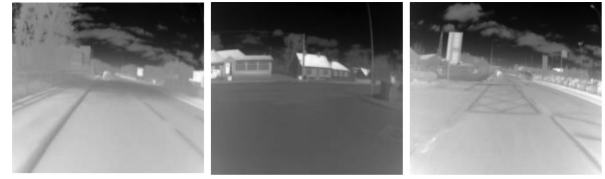
Fig. 7. High-quality thermal frames after applying the shutterless calibration algorithm and image correction methods.
