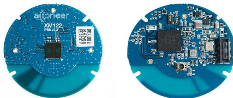
Figure 18: XM122 Aconeer radar sensor module for measuring the object distance.
