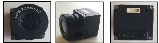
FIGURE 8. Uncooled LWIR prototype thermal camera images from different angles developed under the Heliaus EU project [37].
