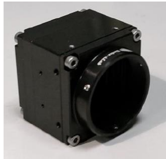
Figure 3: Microbolometer sensor array packaging [49].
