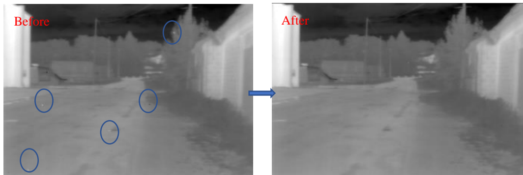
Figure 14: Bad pixel replacement algorithm output on sample thermal frame, left side frame with some bad pixels spotted in blue circles and the right side is processed frame.
