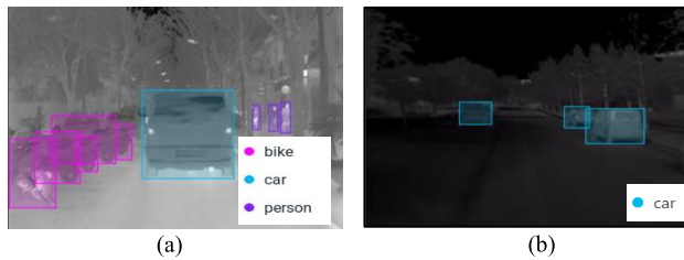
FIGURE 7. Annotated sample images with tight bounding boxes from two different datasets a) CVC-09 dataset sample (road-side view), b) KAIST dataset sample (road-side parking).
