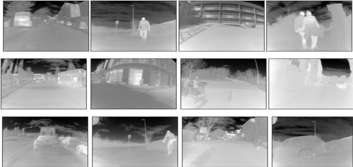
Figure 28: Twelve distinct thermal frames were captured using LWIR 640X480 prototype thermal camera using M-1 and M-2 methods.
