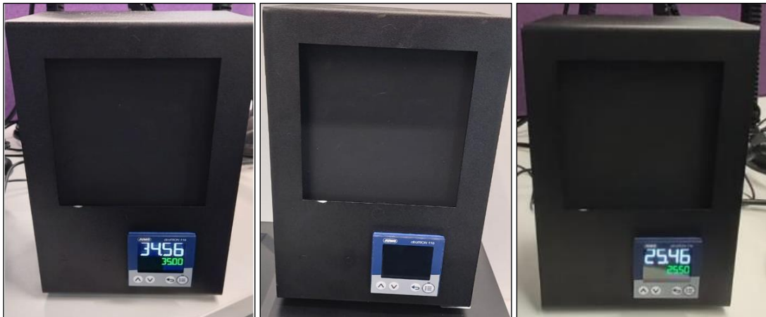
Figure 9: Black body shape for calibrating the thermal camera.
