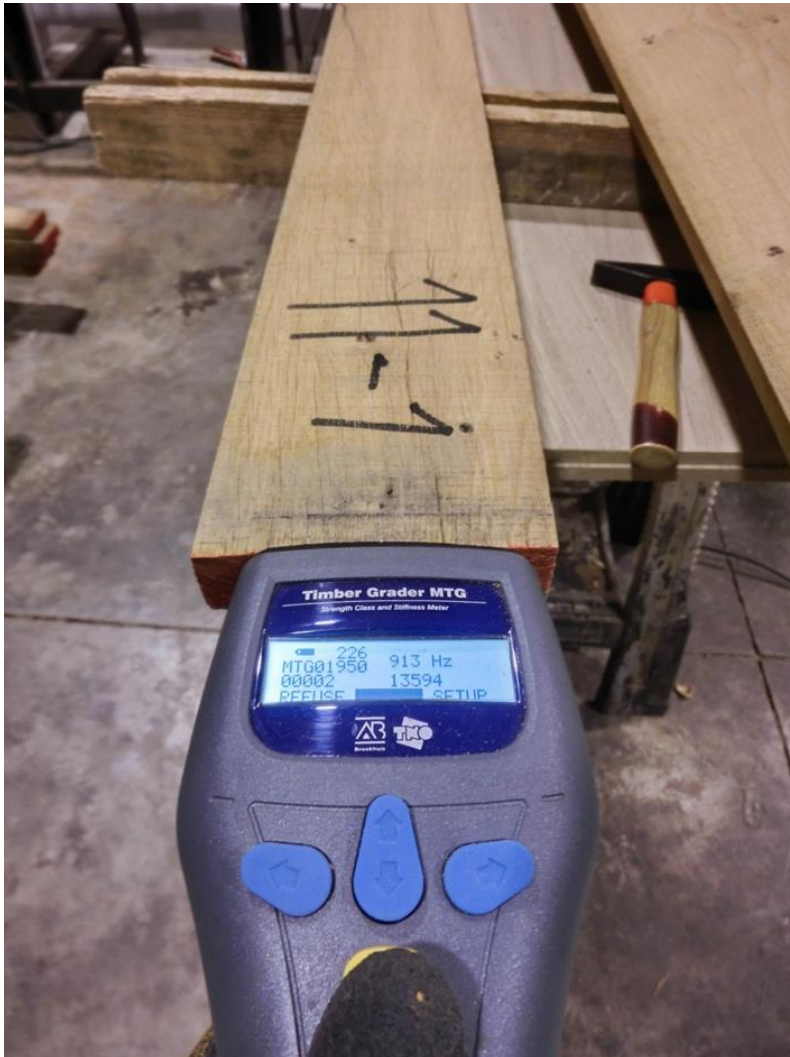
Figure 2-16: Longitudinal vibration testing by MTG
