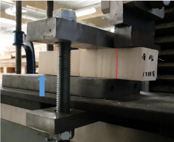
Figure 3-11: Specimen uplift during testing, marked with blue arrow. Glue line marked in red.
