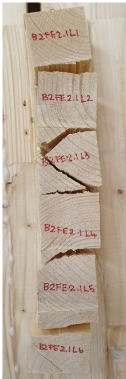
Figure 3-9: Specimen after testing. Failure does not always occur in proximity to glue line.
