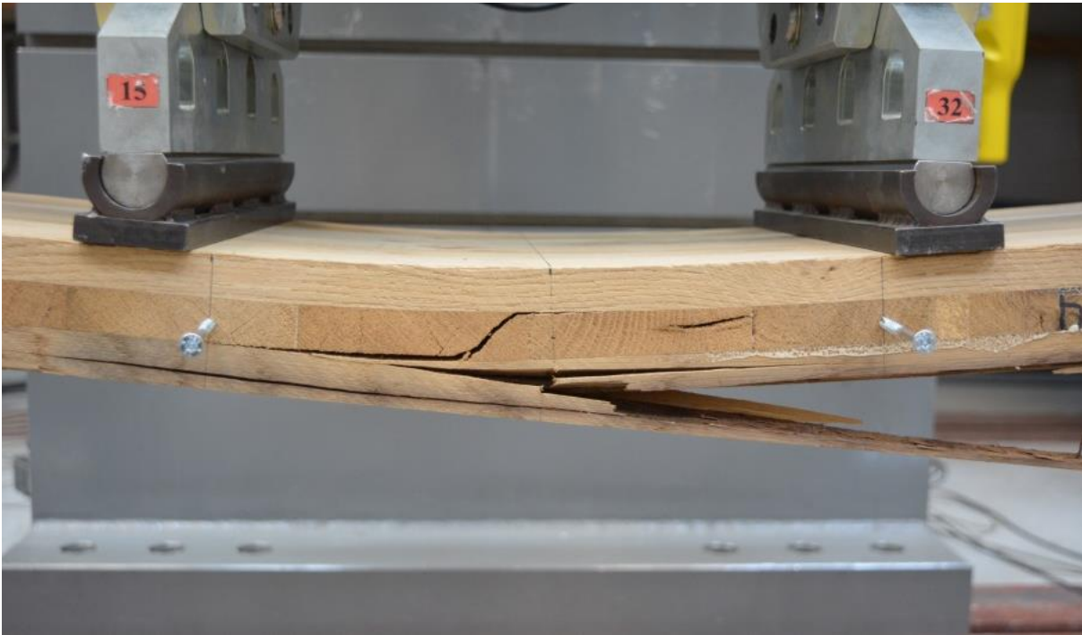
Figure 2-20: RRR CLT panel at failure under four-point bending at 52.20 kN
