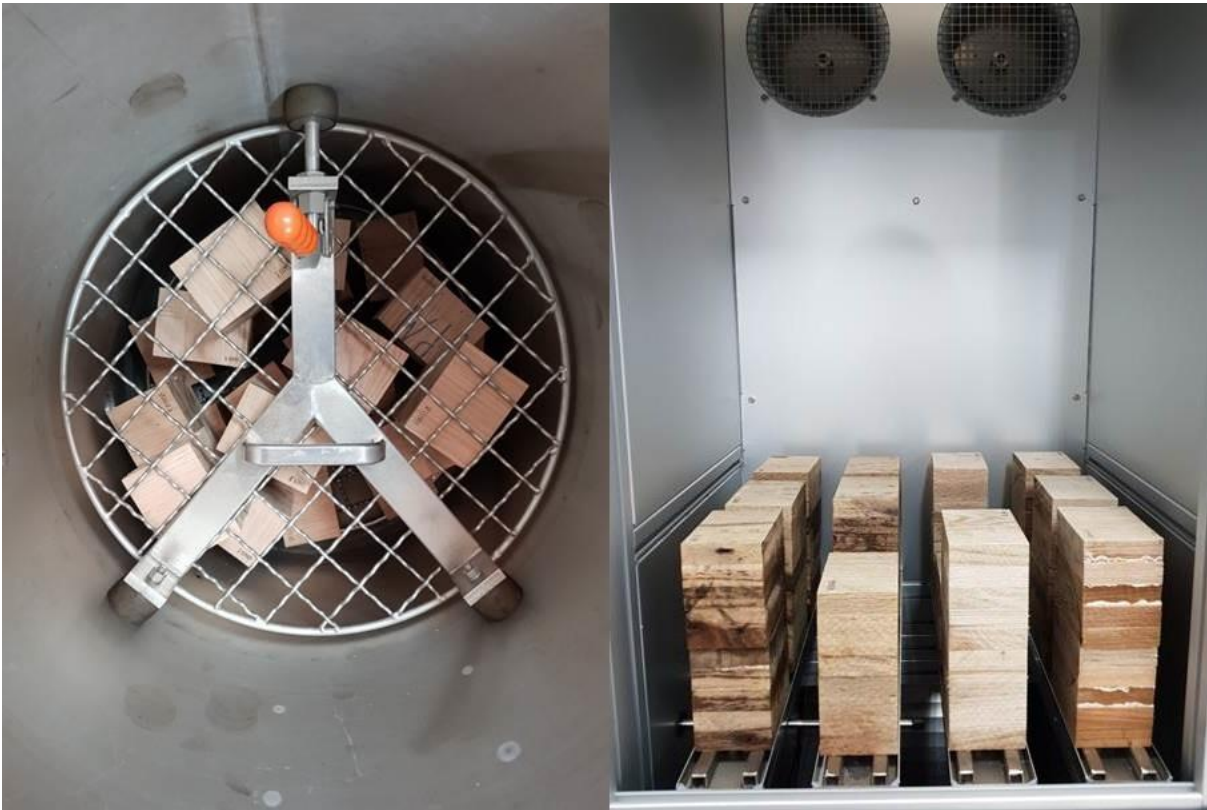
Figure 3-3: Delamination tests of CLT and GLT
