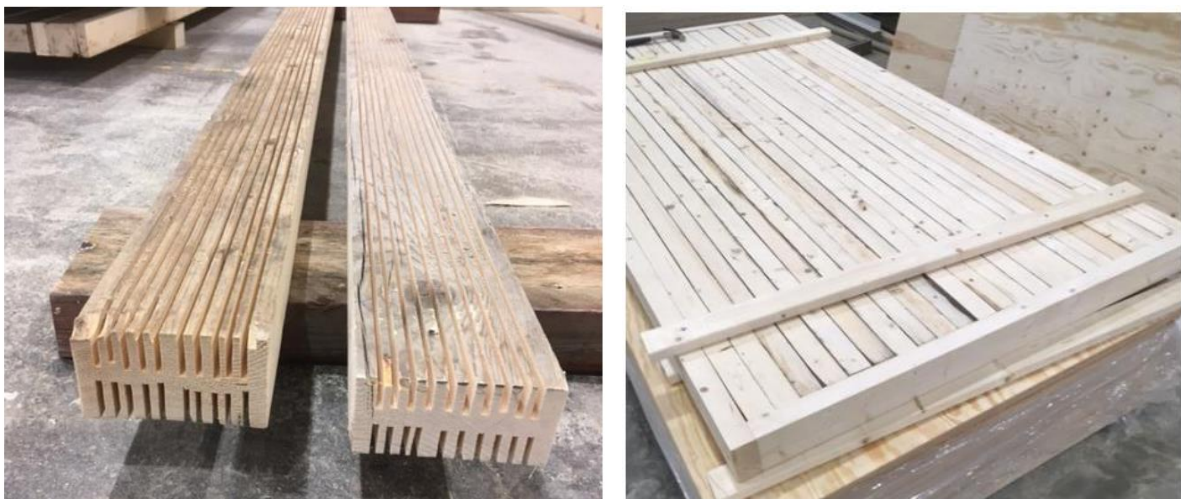
Figure 2-29 Manufacturing of an IsoTimber panel using recovered wood for the uprights (Henriksson 2021).
