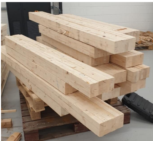
Figure 3-6: Glulam sections after bending test. Sections without bending failure were used for producing shear specimens.
