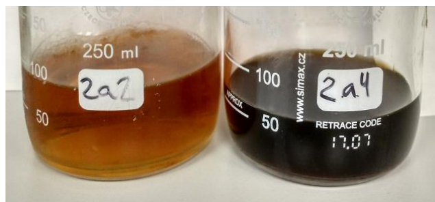
Figure 6.6 Recovered supernatant after enzymatic hydrolysis of pretreated brewery spent grain using 0.80 % of HCl (v/v) at 121.0 °C for 142 minutes with an initial volume of 150 mL of water. The slurry before centrifuging was left overnight at 4.0 °C a pH: 1.0 for the left bottle (golden colour), and 8.0 for the right bottle (dark brown colour)
