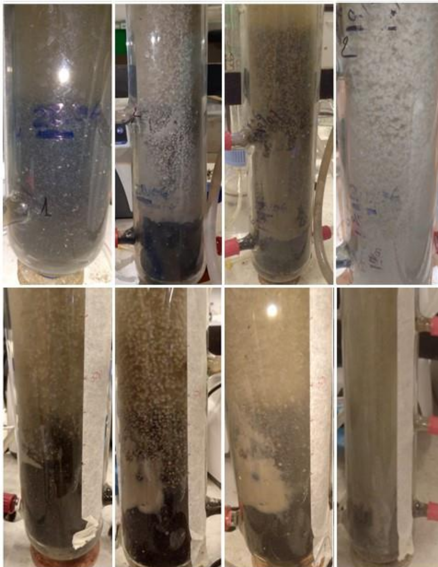
Figure 5.4 Granular sludge development in an EGSB reactor aimed at acidogenesis of brewery spent grain hydrolysate. Fig. 4A – Fig. 4D corresponds to Reactor 1 (R1) and Fig. 4E – Fig. 4H corresponds to Reactor 2 (R2). a) R1 day 0, the fresh granular sludge (inoculum); b) R1 day 9, three different layers in the sludge bed; c) R1 day 19, the granular sludge and the new flocculent sludge prior pH disaggregation; d) R1 day 30, flocculent sludge after the pH disaggregation. e) R2 day 4, granular sludge and new flocs; f) R2 day 13, three layers within the sludge bed; g) R2 day 16, granular sludge and flocs after natural disaggregation; and h) R2 day 40, two different layers in the sludge bed with granular sludge at the bottom and flocculent sludge on top
