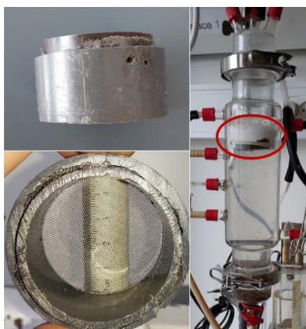
Figure 7.2 Sectional tube with a titanium mesh with a pore size of 1 mm, and placement inside of the upflow anaerobic sludge bed reactor
