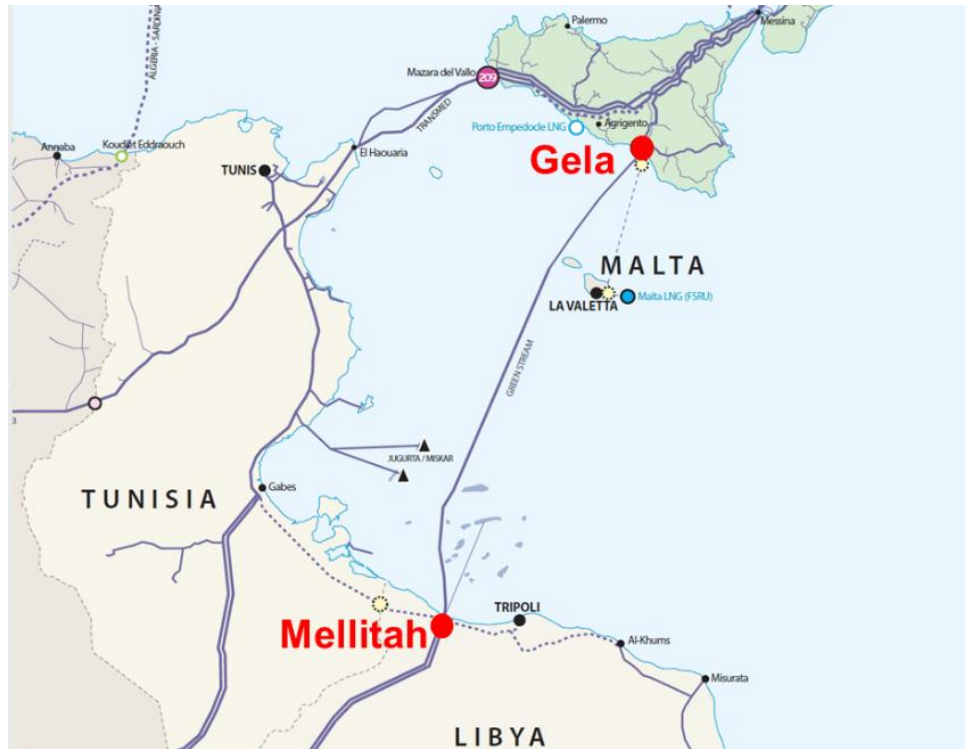
Figure 4.1. Mellitah and Gela gas terminals are connected by the 520-km Greenstream subsea natural gas transmission pipeline [137]
