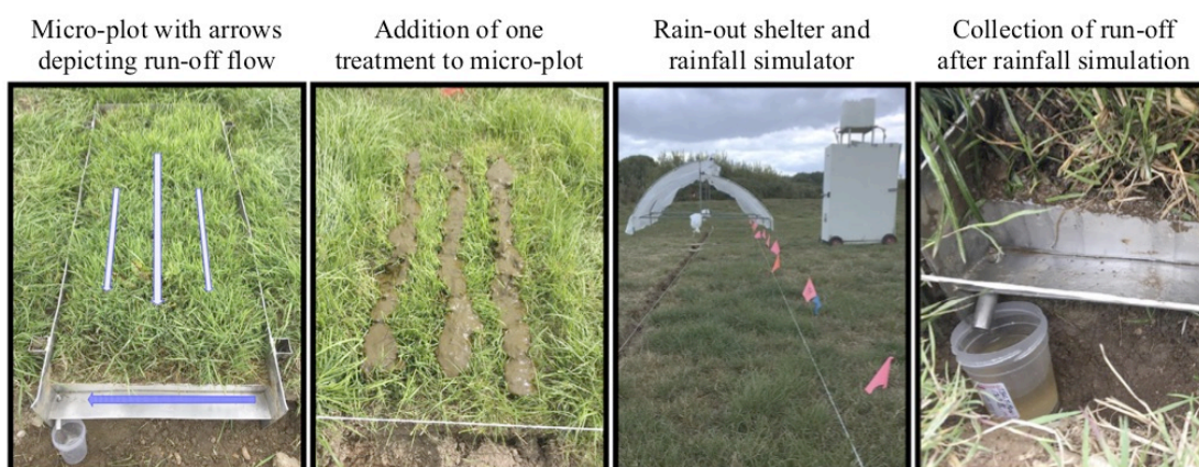
Fig. 1. Depiction of experimental set-up, using micro-plots ( 40 \times 90\text{ cm} ) to which different treatments (slurry or digestate) were applied before plots were subjected to a number of rainfall simulation events, where specialized frames allowed collection of runoff water.
