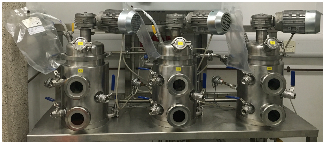
Figure 4.1 – Triplicate 10 L continuously stirred tank reactors (CSTRs)
