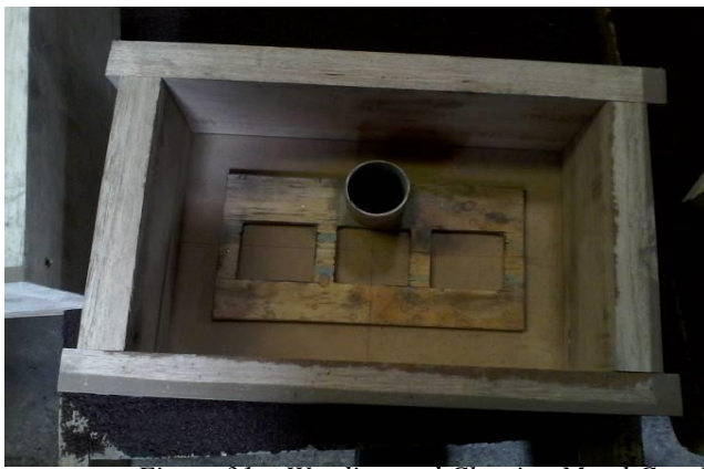
Figure 31a: Weeding and Clearing Metal Cast Prototype and Weeding Flat Blade Cast Mould
