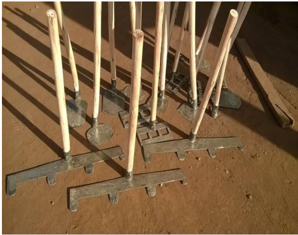
Figure 5-3: 3 Blade Planter Mould and Metal Cast Prototypes
