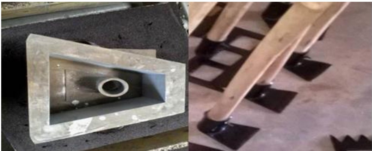
Figure 4-21: Sasakawa Planting Hoe Mould and Metal Cast Prototypes
