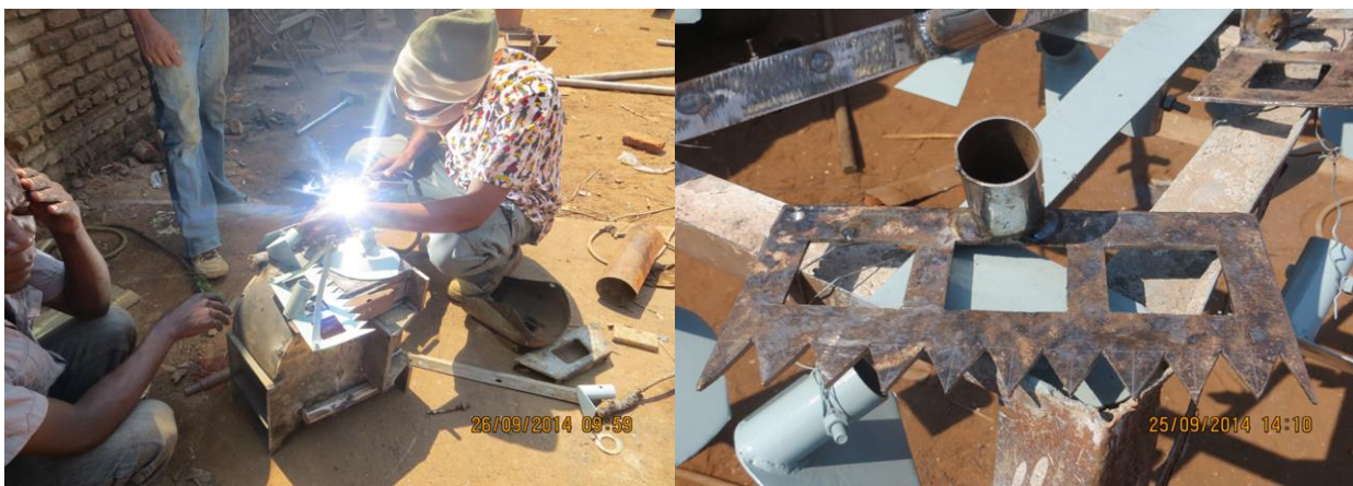
Figure 7b: A local artisan welds pieces of scrap metal to produce prototypes for on-farm testing.
