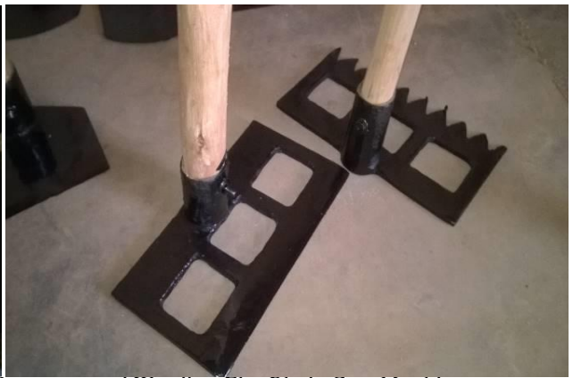
Figure 31a: Weeding and Clearing Metal Cast Prototype and Weeding Flat Blade Cast Mould
