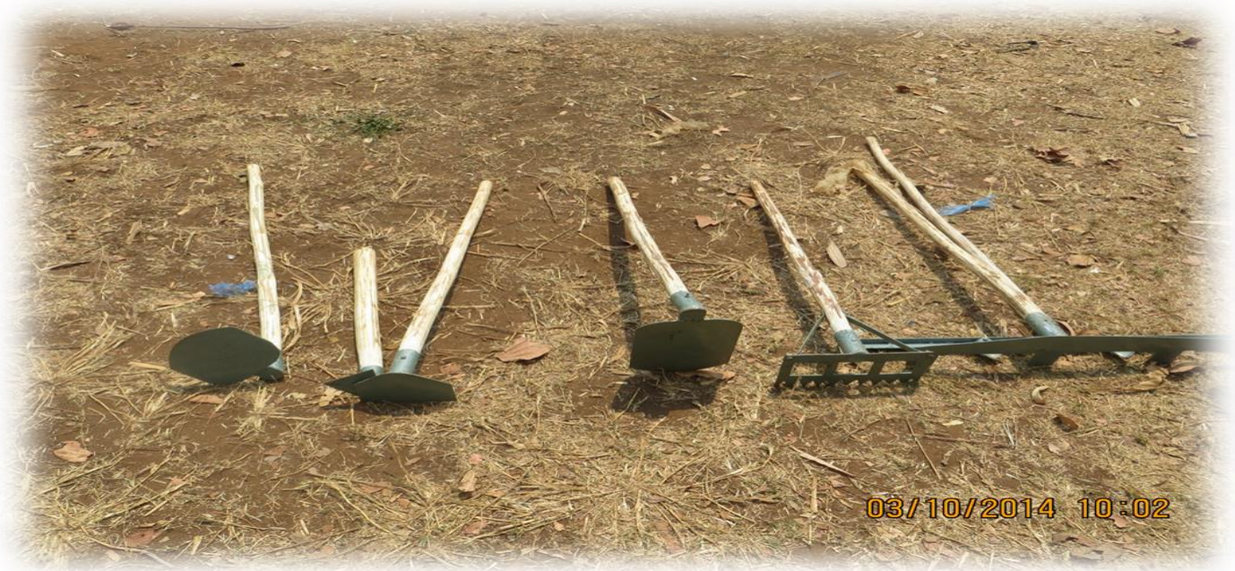
Figure 5-1: Welded cultivation prototypes co-designed with women farmers.
