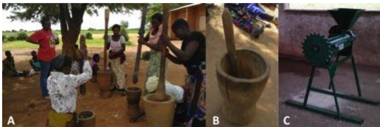
Figure 5-5: Maize grinding: traditional methods versus new prototype.
