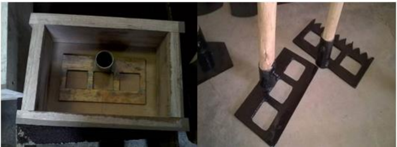
Figure 4-20: Weeding and Clearing Prototypes and metal cast Mould
