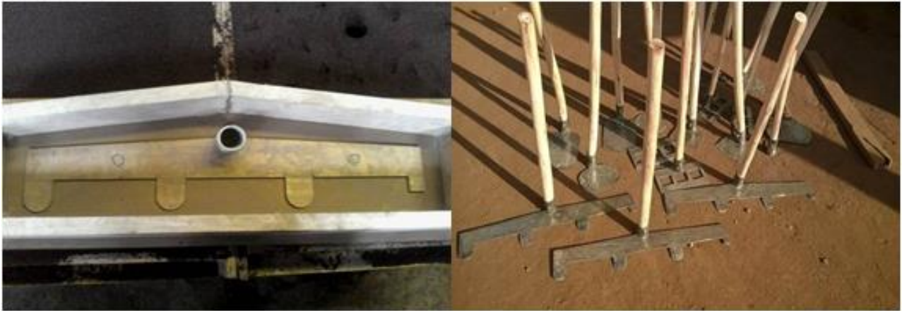
Figure 4-19b Blade Planter Mould and Sample of Metal Cast Prototypes
