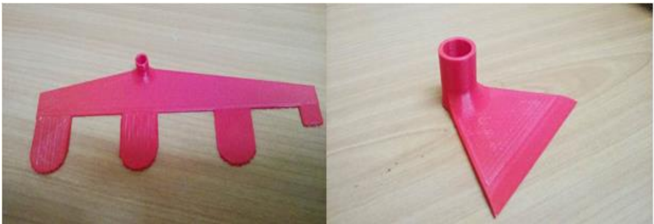
Figure 4-10: 3-Blade Planter & 1-Seed Sasakawa 3D Printed Micro Prototypes.
