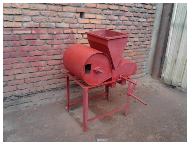
Figure 5-7: Soya thresher and Winnower Co-Designed Prototype
