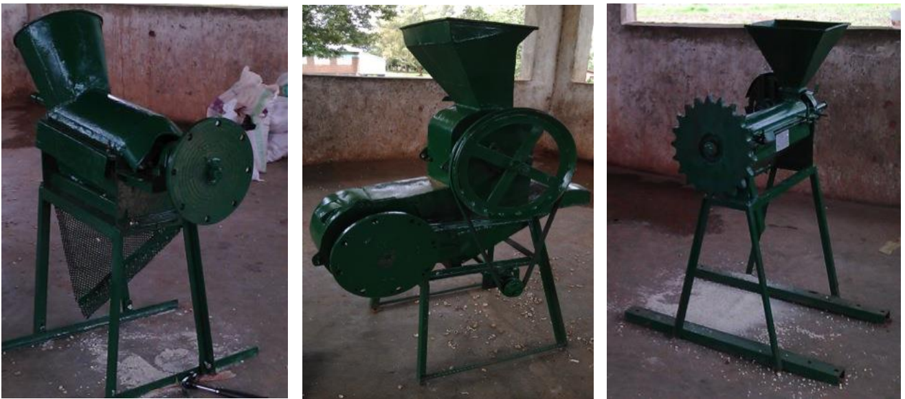
Figure 25a: Prototypes (scrap metal): 1) Maize Sheller, 2) Groundnut Sheller & Winnower, 3) Maize Grinder
