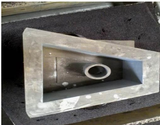
Figure 31b: Sasakawa Planting Hoe Mould and Metal Cast Prototypes
