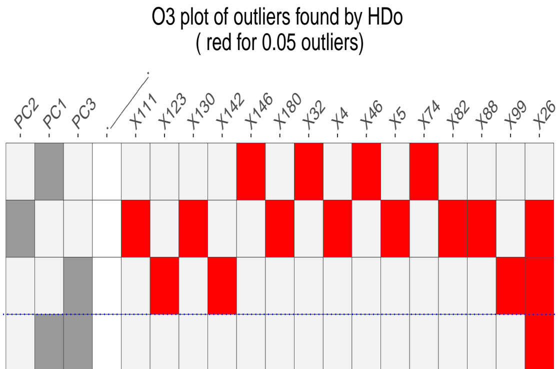
Figure 4.18: O3 plot of case study data. Each row represents the combination of variables for which at least one outlier was found; dark gray colour represents the presence of the variable in the combination. Red cells are the outlying data point with corresponding individual ID represented by X^*
