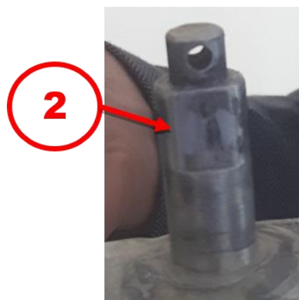
Figure A.5: Image showing wear on the blade shaft, particularly at the corners.
