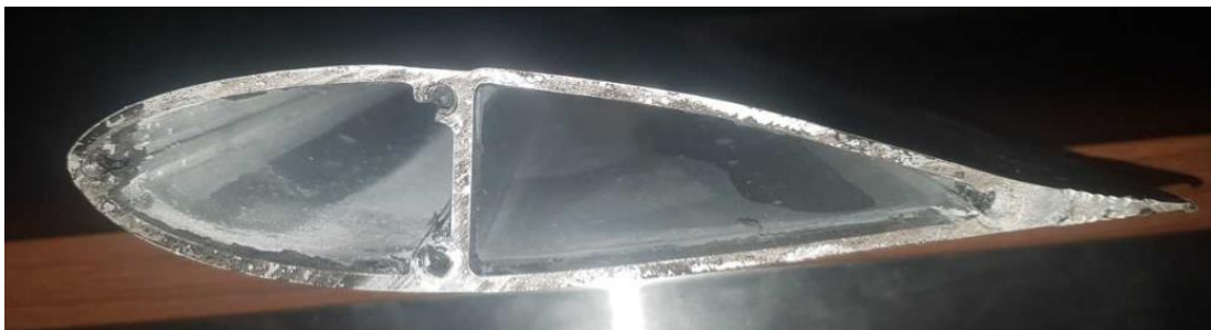
Figure A.19: Existing blade cross section showing shear web support.
