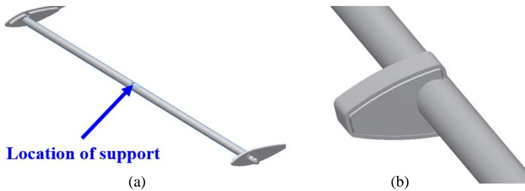
Figure A.18: New blade design showing mid-blade support
