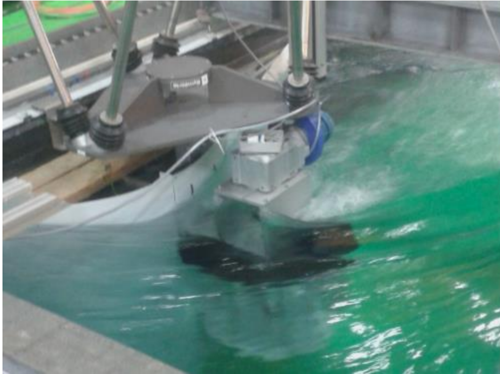
Figure 7.2: Image of the 1:20 scale device being tested in IFREMER’s flume tank, with turbine positioned at mid-depth.
