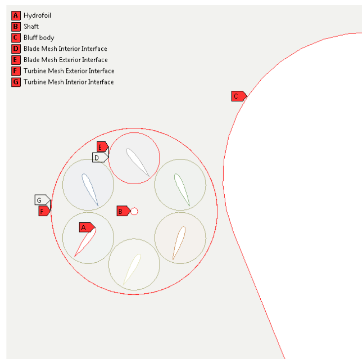
Figure 7.1: Schematic showing the arrangement of the model meshes with key components identified.
