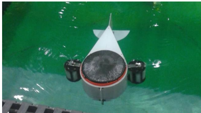
Figure 4.3: 1:40 scale device tested at IFREMER.
