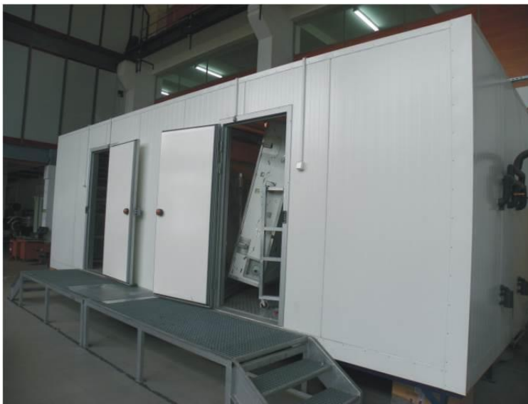
Fig. 9. General view of calorimetric hot box.
